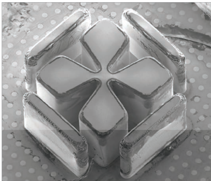
Electroformed four-spring self-centring fibre alignment structure in nickel.
